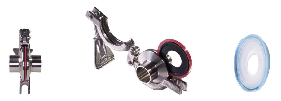
Fluid Path's innovative outer ring geometry provides the hands-free benefit that flanges generally offer, but the 180° of spacing allows the gasket to slide into place without requiring installers to spread the piping apart beyond what it was designed to be separated. System builders can assemble skids without special consideration for difficult flanges and other gripping gaskets.
