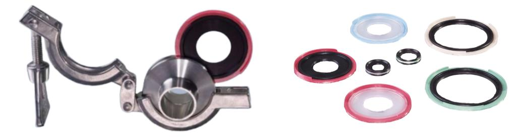
Fluid Path Products has engineered the highest-performing sealing gaskets available. The ridged plastic outer ring prevents the elastomer seal from being over-compressed into the processing pipeline. The outer ring acts as a stop to ensuring a seamless transition in piping connection and creating a pipeline that is free of entrapment.
