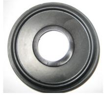
Competitor A: Gasket deformed and extruded .150 into the pipeline, large sections stuck to the ferrule faces.
