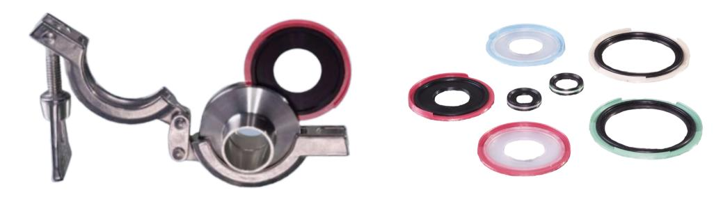
Fluid Path Products has engineered the highest-performing sealing gaskets available. The ridged plastic outer ring prevents the elastomer seal from being over-compressed into the processing pipeline. The outer ring acts as a stop to ensuring a seamless transition in piping connection and creating a pipeline that is free of entrapment.
